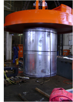
Fig: 3 – 2000mmØ CFLD Lifting 5 ton core
